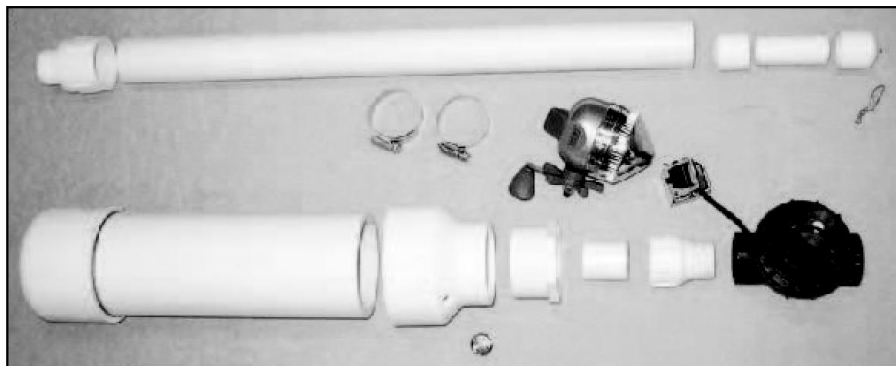
Figure 4 — The spudgun is easy to fabricate from the pieces shown.
